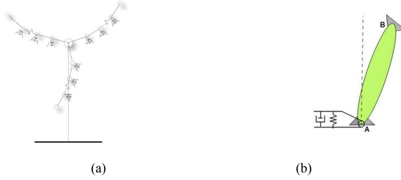
Fig 2: Modeling of structural rigid beam,(a) For entire model,(b)For each elements [40]
