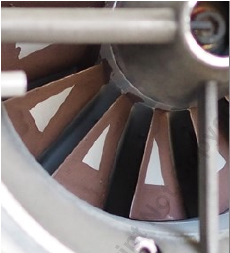
Fig. 2 Simulated fouling pattern in test rig compressor
