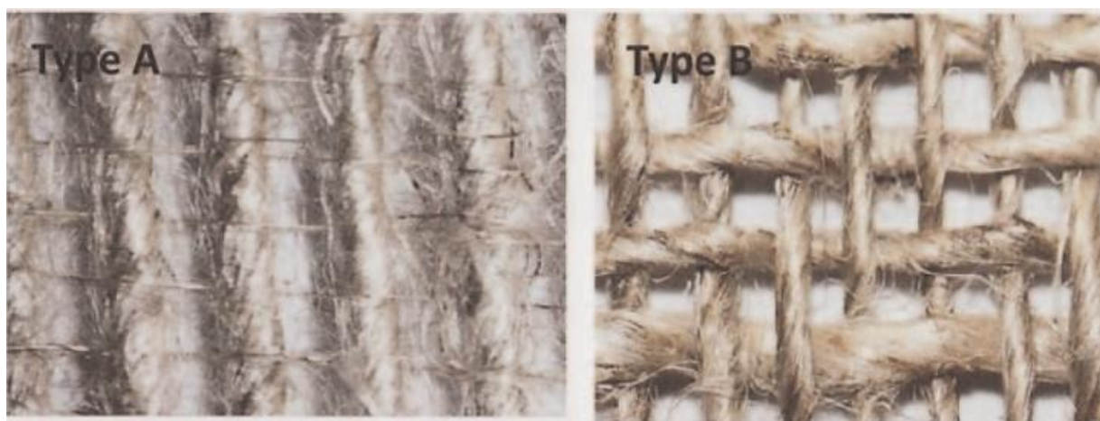
Figure 11. Weave architecture types: (A) plain; (B,C) two different twill; and (D) dobby [75]. Adapted with permission from [17]. Copyright 2013 by SAGE.
