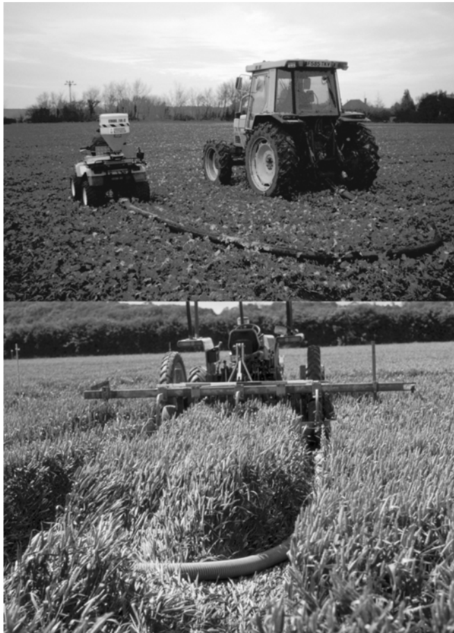
Fig. 6. Umbilical hose trials
