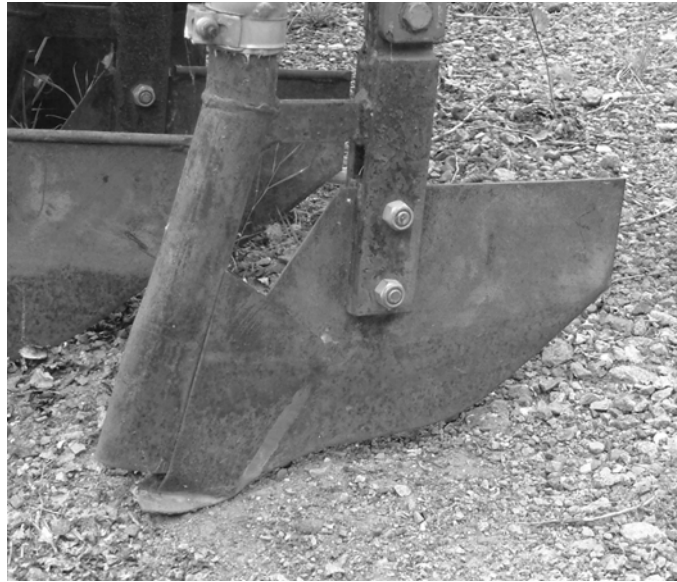
Fig. 2. Single piece tine with leg profile III and 40 mm wing or single piece tine (S5)
