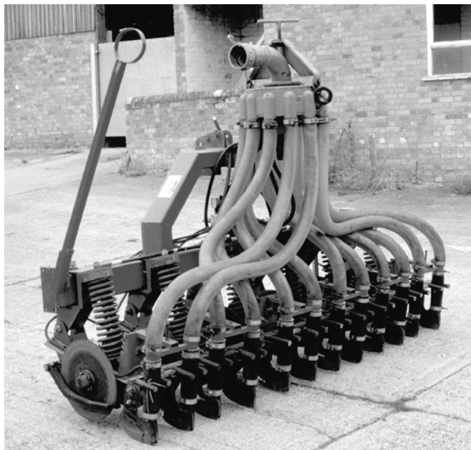
Fig. 5. General layout of implement onto which shallow I injector tines (C2) were attached
