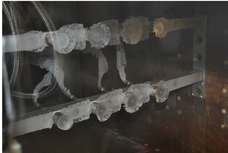
Figure 2: Mode I test rig in place in the test section of the CIWT
