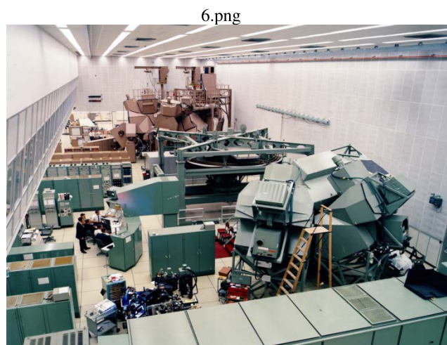
FIGURE 5. The physical twin of Apollo 13, the green side is the foreground simulator, and the brown side is the Command Module Simulator [2].
