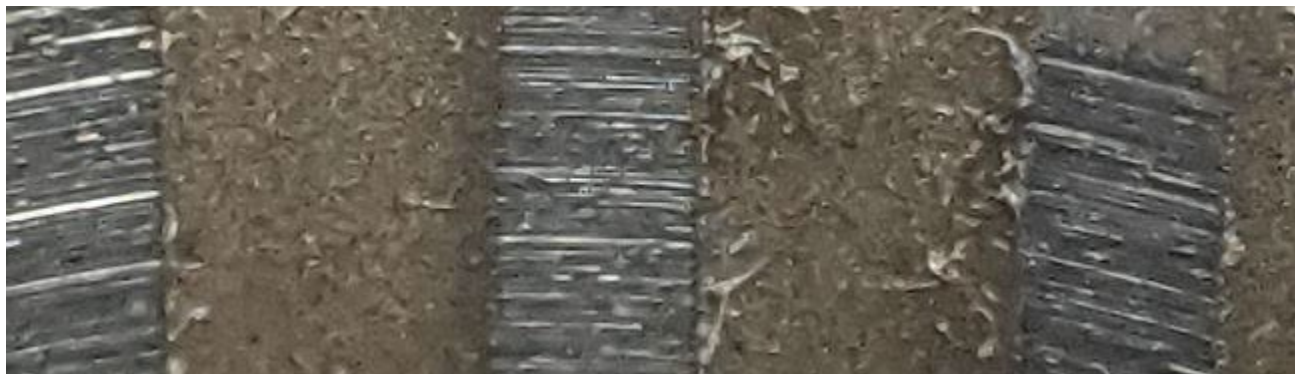
Figure 13. Photograph of an unfired insert showing grooves on the landings from machining.
