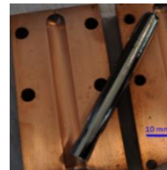
Fig. 1. MG rod ( Zr_{55}Cu_{30}Ni_{15}Al_{10} , about \varnothing 10 mm, 100 mm long) produced at Cranfield University by tilt casting into a copper mould.
