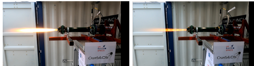
Figure 3. Hot-fire testing (E-300) with 12 s burn time. Stabilised flow with Mach diamonds (right), performed at NTP conditions with Protolaunch test bed.
