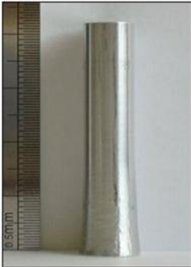
Figure 13 Photographs of the post-test geometry for the AA 7010 Taylor specimen after impact at 200 m/s
