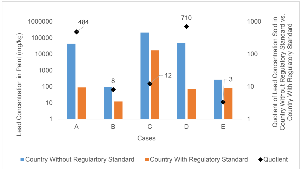
Figure 4 Lead levels in paints of the same brand and same colour being sold in developing countries with no regulatory standard vs. those sold in developing countries with voluntary regulatory standards (data source: (Betne et al. 2011))
