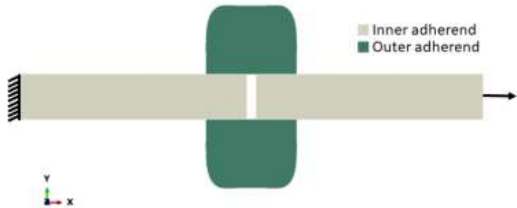
Figure 5 analysis setup for tensile loading condition
