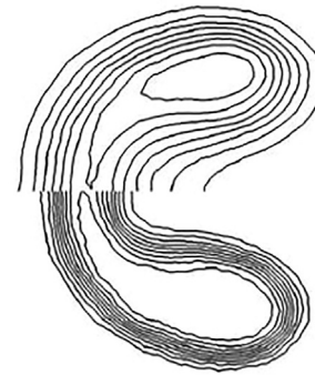
FIG. 9. Helium bubble shape in terms of volume fraction isovalues. Comparison between DG^3 (top half) and DG^1 (bottom half) resolution. [Adapted with permission from E. Franquet and V. Perrier, “Runge-Kutta discontinuous Galerkin method for the approximation of Baer and Nunziato type multiphase models,” J. Comput. Phys. 231 , 4096–4141 (2012). Copyright 2012 Elsevier Ltd.]
