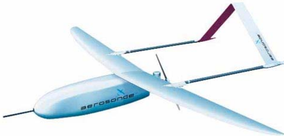
Figure 9-26 The Aerosonde UAV – a representative vehicle for the aerial communications subsystem (Aerosonde, 2000).
