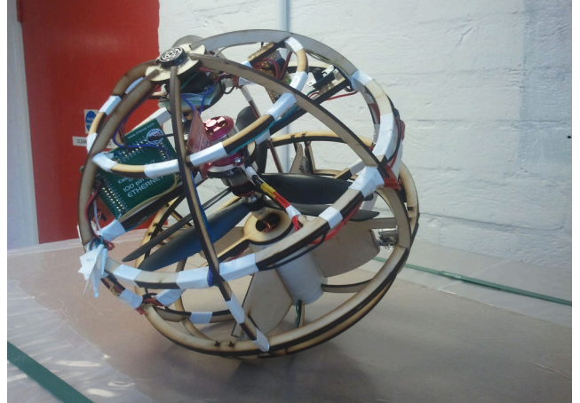
Fig. 14. The completed flight ready spherical UAV.
