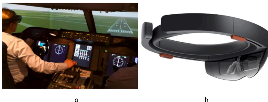
Fig. 1. The cockpit display systems on flight simulator on the scenario of instrument landing (1a); participant wears the head-mounted display Augmented Reality device (HoloLens) during the experiment (1b).
