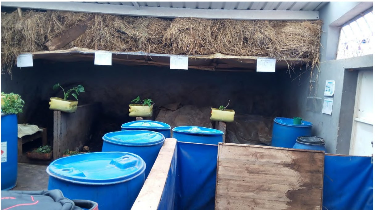
Figure_Apx E-4 Loowatt composting site (rice straw storage area and small windrow composting below. The blue drums contain digestate
