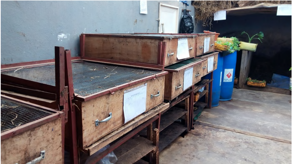
Figure_Apx E-5 Vermicomposting drawers in Loowatt treatment site
