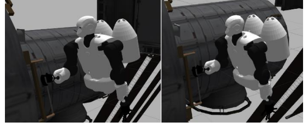
Fig. 1. Humanoid robot grasping a ISS handrail
