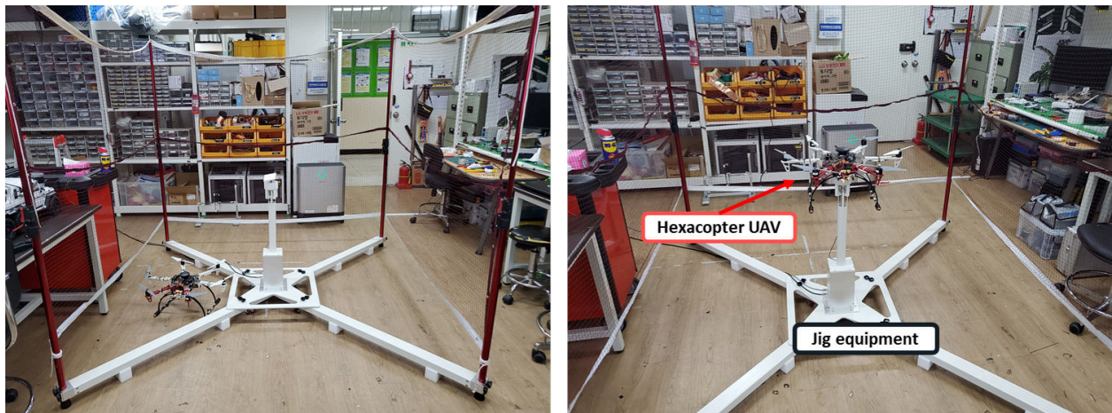
Fig. 8 The actuator FDD method test using the jig equipment
