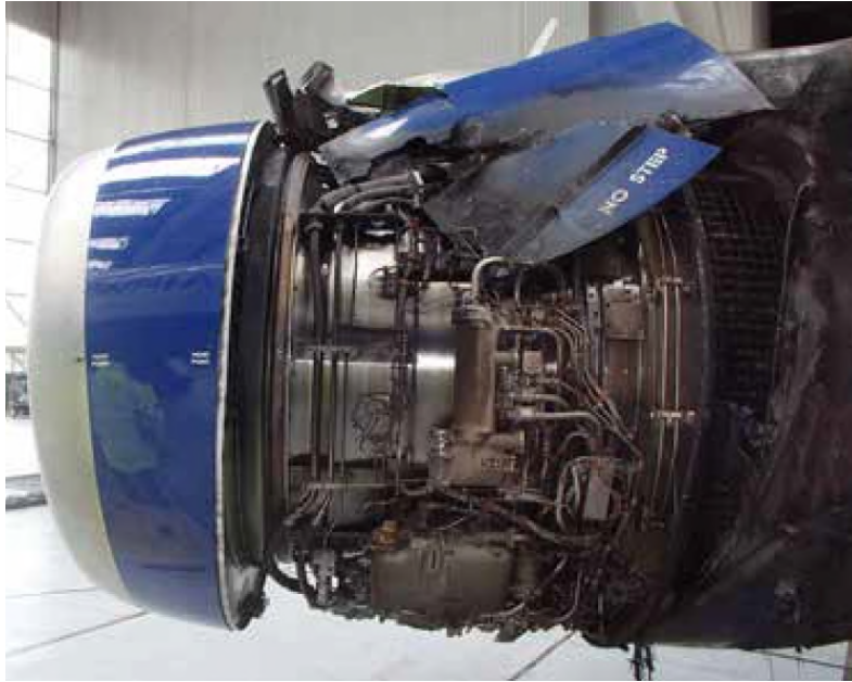
Figure 3. Remaining parts of the right-hand engine inboard FCD of the British Airways Airbus A319-131 G-EUOE following the 24 May 2013 accident (photograph reproduced from the AAIB Aircraft Accident Report 1/2015 (AAIB, 2015)).
