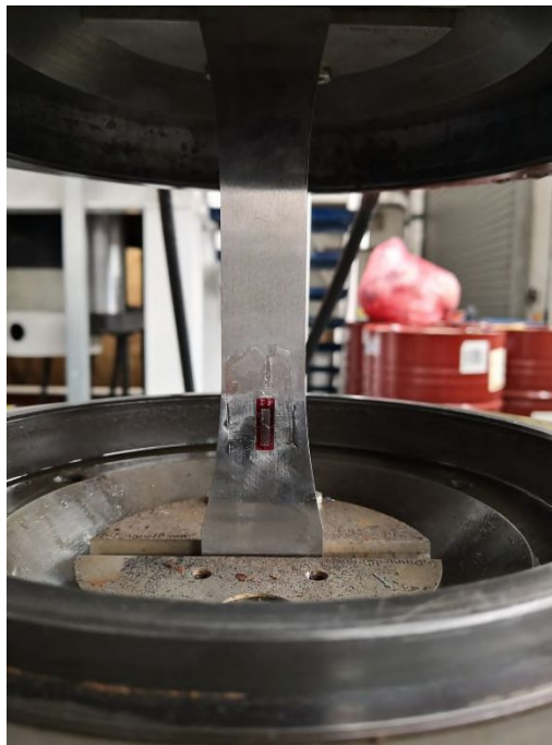
Figure 34 - Uniaxial fatigue specimen undergoing fatigue testing
