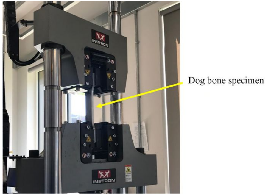
Figure 15 - Dog bone specimen undergoing pre-tensioning
