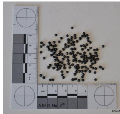
Figure 2. Typical examples of the ball bearings recovered from the M75 Yugoslavian grenades.
