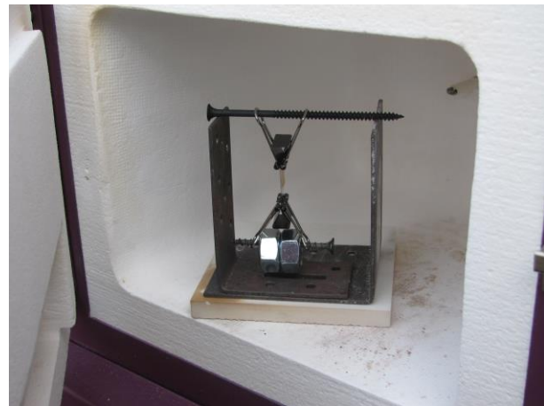
Fig. 15: Thermomechanical Demise Test Set-Up
