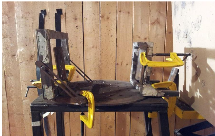
Figure 1 Target arrangement showing (from left to right) moveable front plate holder, rear plate holder and strawboard witness pack.
