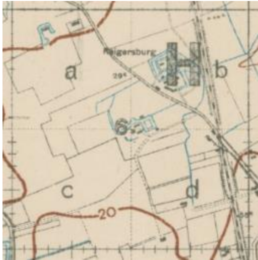
Figure 5-2 A numbered square showing the subdivision into smaller areas a, b, c, d with scale markings on the side (Adapted from War Office, 1917b)
