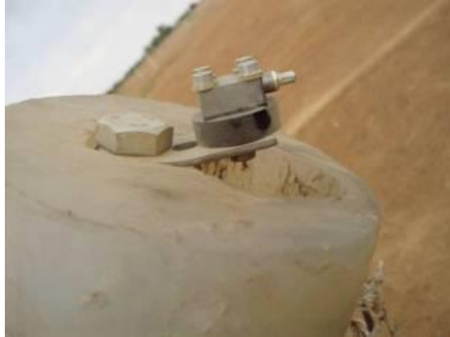
Figure 85: Photograph of damaged triaxial head accelerometer.
