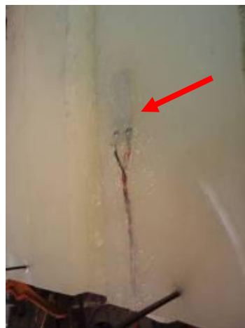
Figure 71: Photograph of the abdominal insert prior to casting the outer layer of the SATS with the back PVDF transducer.
