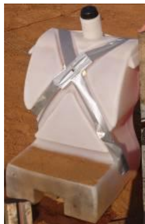
Figure 20: Photograph of a SA Waterman torso surrogate with a transducer package mounted on the chest area.
