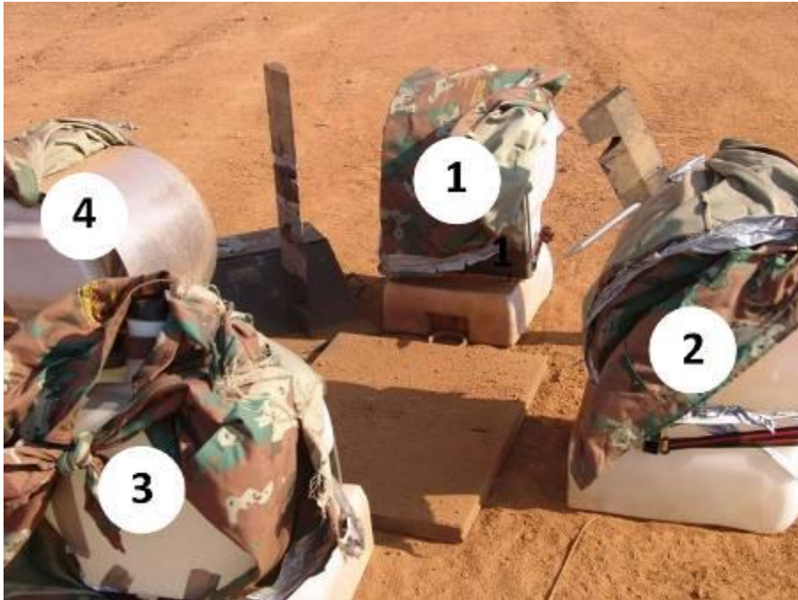
Figure 57: Photograph of the four SA Waterman Surrogates and pressure probe after the test (1. Foam; 2. Lexin; 3. Uniform Only; 4. Aluminium Sheet).
