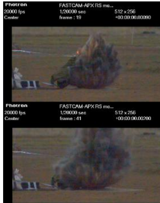
Figure 91: Still frames of the camera footage from the blast at 0.9 ms (left) and 2 ms (right).
