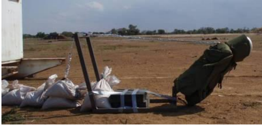
Figure 76: Photograph showing the positioning of the SATS (wearing protective clothing) and the stand in relation to the AP mine and the splinter proof shelter.
