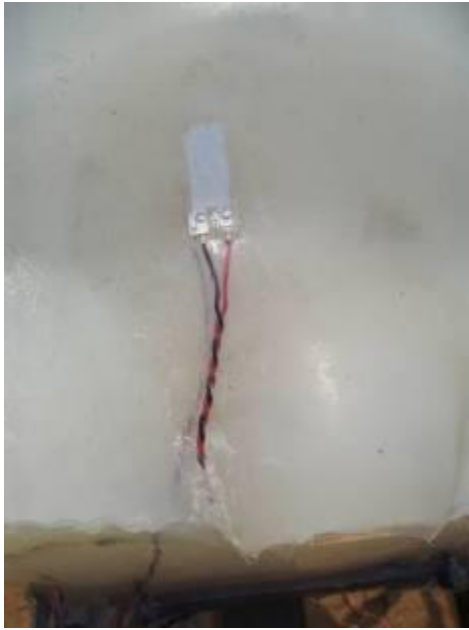
Figure 72: Photograph of the abdominal section of the SATS, after casting the outer layer, with the front PVDF transducer positioned (above the top of the middle PVDF transducer that cannot be seen here).
