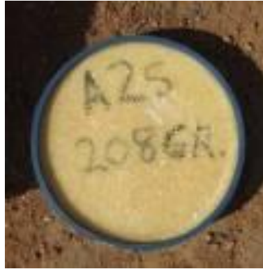
Figure 9: Photograph of an AP blast mine surrogate (208 g pentolite charge).
