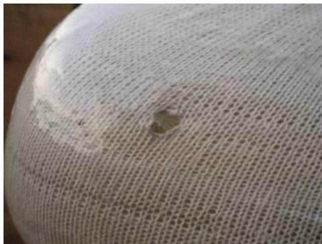
Figure 84: Photograph showing a penetration of the Mutton cloth layer by a small stone on the right shoulder of the SATS.
