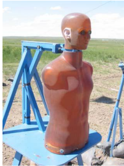
Figure 67: The Mannequin for the Assessment of Blast Incapacitation and Lethality (MABIL) developed by Defence R&D Canada, Valcartier [Bouamoul et al. : 2007].
