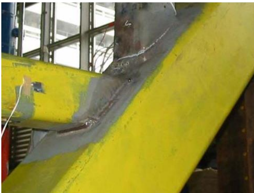
Fig. 6 The final failure of SHS K-joint
