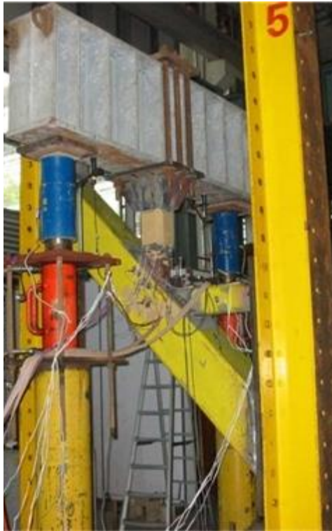
Fig. 2 The experimental test rig for cracked SHS K-joint
