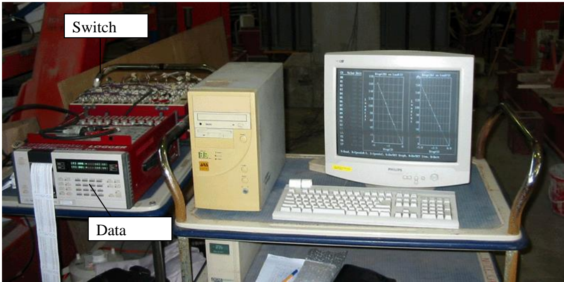
Fig. 4 The recording system set-up used during the test process
