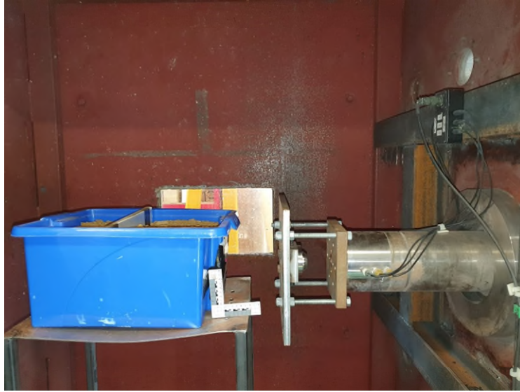
Figure 4 Experiment setup for gas gun firings into sandbag target with Aluminium plate at 226mm from point of impact
