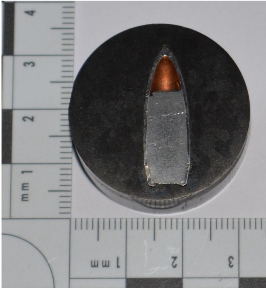
Figure 4.2 Mounted section of 7.62mm projectile. Mean core hardness 7.8Hv (SD 0.6Hv, n = 3), lead mixed with antimony. Mean jacket hardness of 184.4Hv (SD 12.3Hv, n = 3), steel with internal and external copper washes [12].
