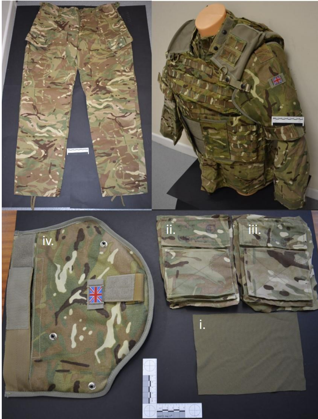
Figure 5.1 Examples of MTP clothing used – clockwise from top left: MTP trousers; top right: t-shirt, UBACS, smock, and brassard as worn by service personnel; bottom: i. t-shirt, ii. UBACS, iii. smock and iv. brassard layers prepared for testing. Laundering detail and fabric analysis data for this clothing used within these experiments is detailed in previously published work [29]
