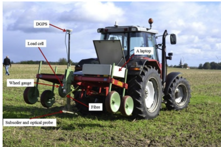
Figure 1. The multi-sensor platform for the on-line measurement of soil properties
