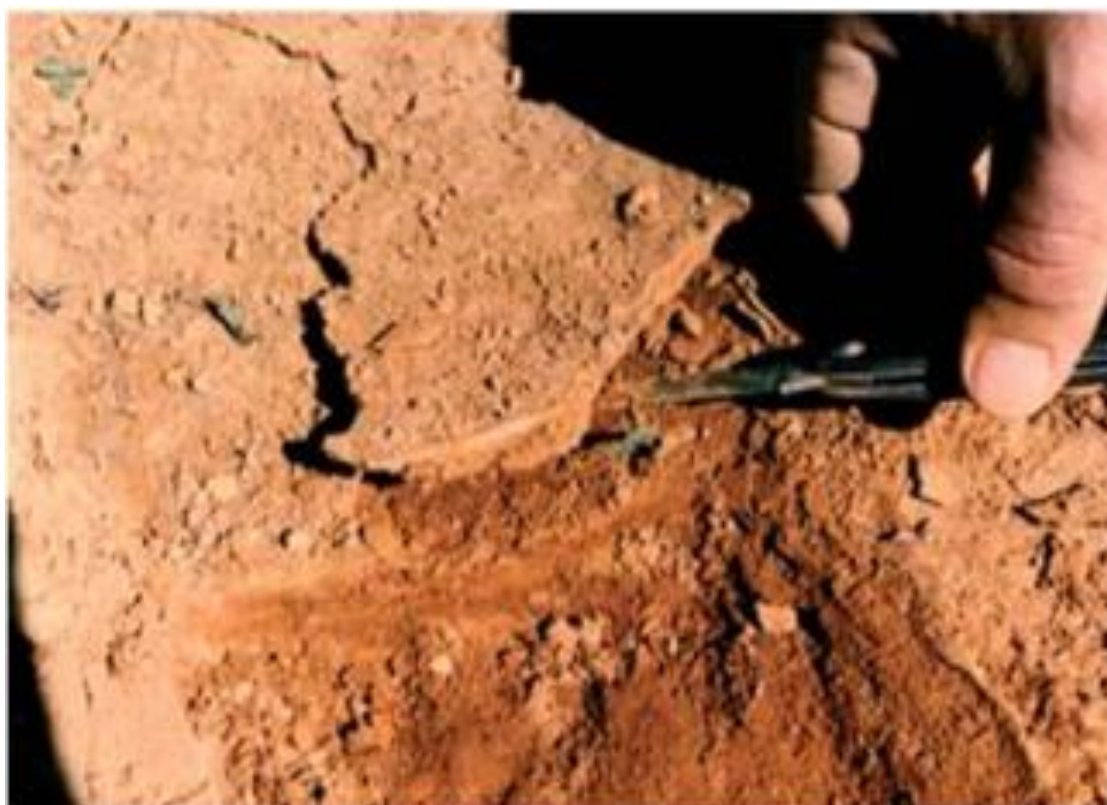
Figure 2-8 A thin surface crust caused by raindrop impact on a bare soil of poor structure (after, Shaxson and Barber, 2003).
