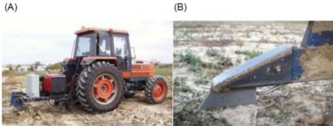
Figure 2-19 On-line air permeability measuring system to estimate soil compaction (A) and the subsoiler with the outlet holes plate attached (B) (after, Stombaugh, 2014).
