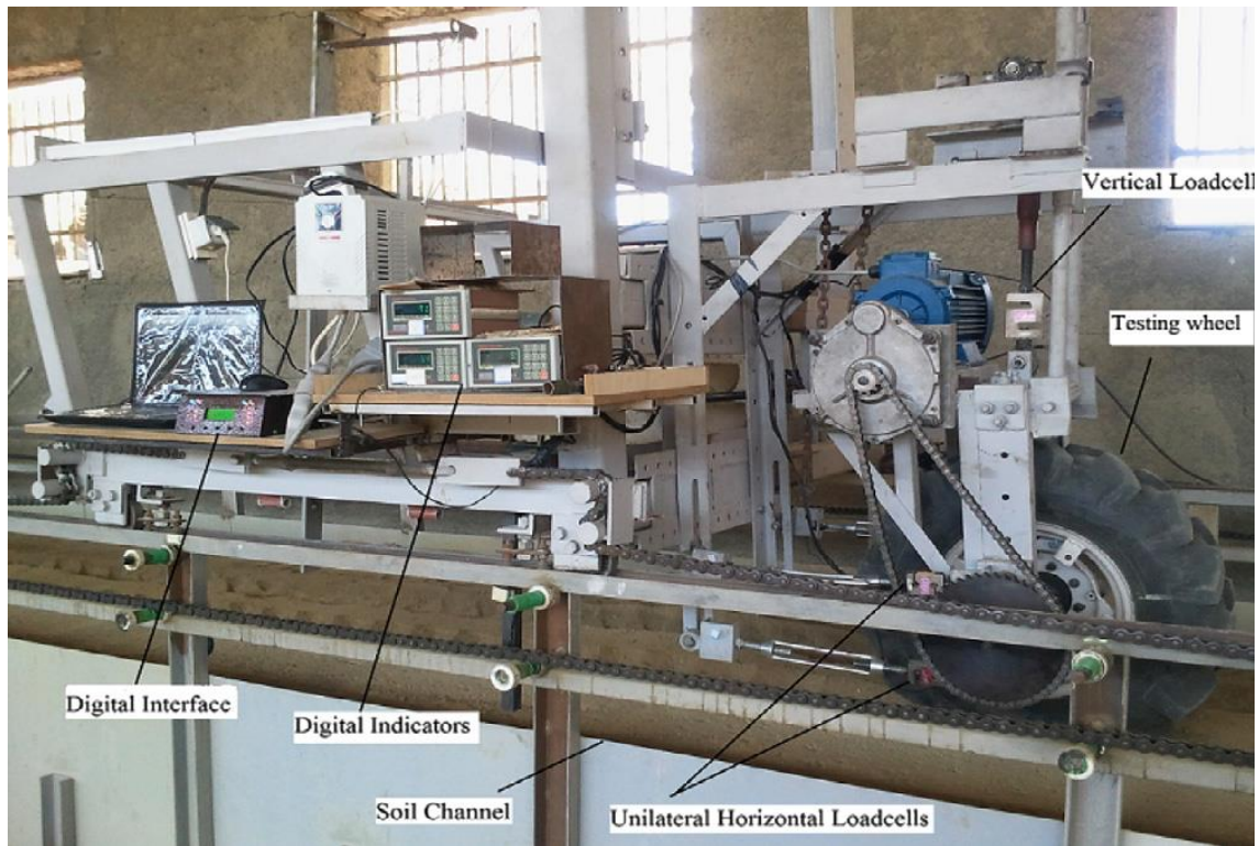
Figure 2-5 Single wheel testing system of soil compaction in a soil bin. (after, Taghavifar and Mardani, 2014).
