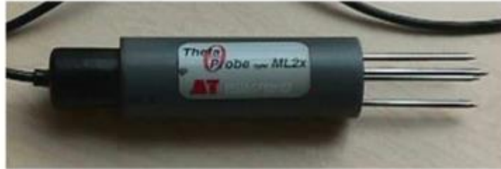
Figure 2-16 ThetaProbe soil moisture sensor. The four stainless steel electrodes are 6 (cm) in length and 3 (mm) in diameter (after, Kaleita et al., 2005).
