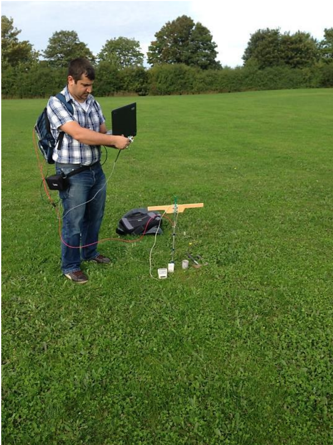
Figure 3-15 The prototype of the field measuring system of volumetric moisture content ( \theta_v ), gravimetric moisture content ( \omega ) and bulk density (BD) carried in a rucksack.
