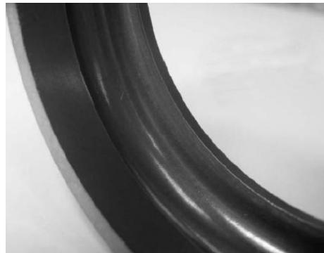
Fig. 91: Detail of bearing outer race after one month
