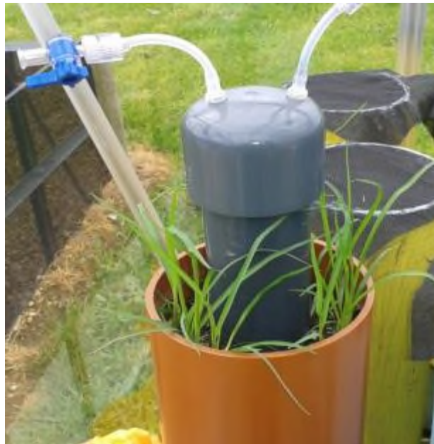
Figure 4-2 Headspace chamber in planted pot showing gastight inlet and outlet ports and luer lock valve
