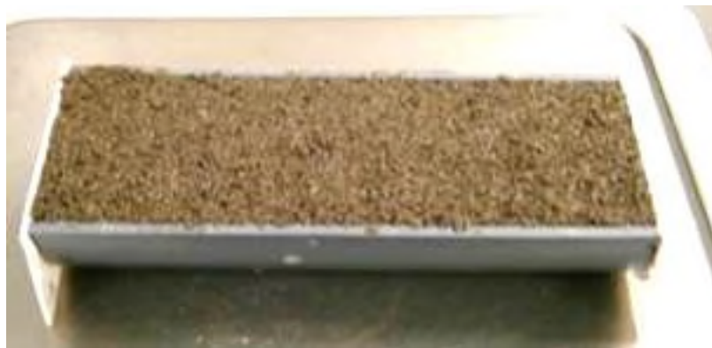
Figure 3-2 Incubation microcosm packed with soil
