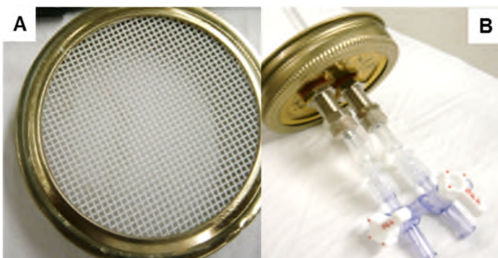
Figure 3-3 (A) Lid with plastic mesh for incubation and storage (B) Airtight lid with inlet and outlet for respiration measurements and air sampling
