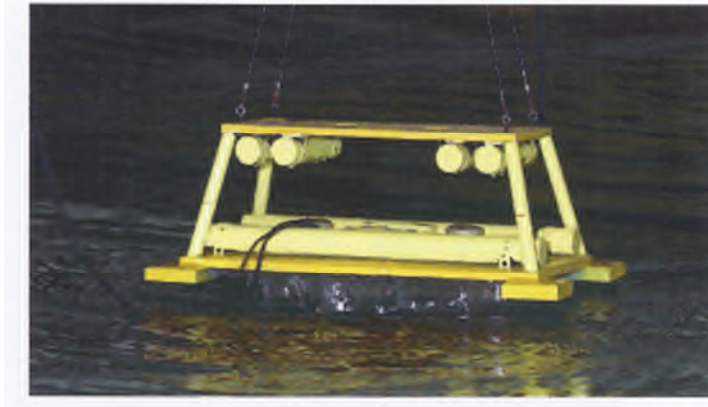
Figure 2-9 Model of a subsea structure in the phase 1 of the test
