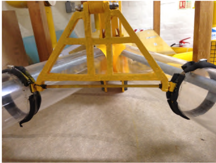
Figure 5-23 Lift Frame linked to the demonstrator
