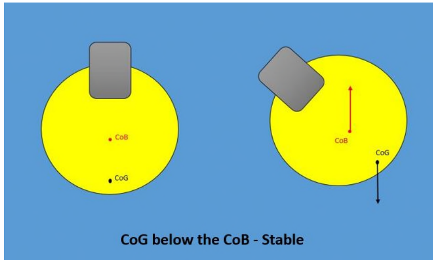
Figure 2-4 Submarine Stability - Stable State
