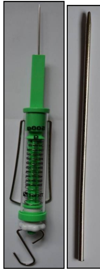
Figure 9 - Completed pocket penetrometer and detail of probe with flat tip at base and 30° at the top.
