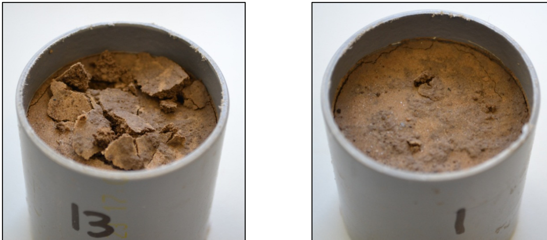
Figure 11 - Photograph of S2 samples after flat probe (left) and pointed probe (right) penetration
