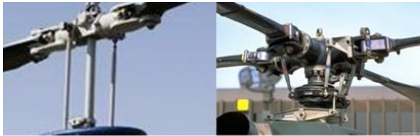
Figure 3-23 Bell206L-4 and MBB Bo105 main rotors
