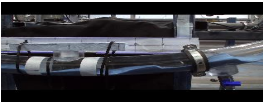
Figure 5-25: Sand dune reach stability at water velocity =0.18m/s
