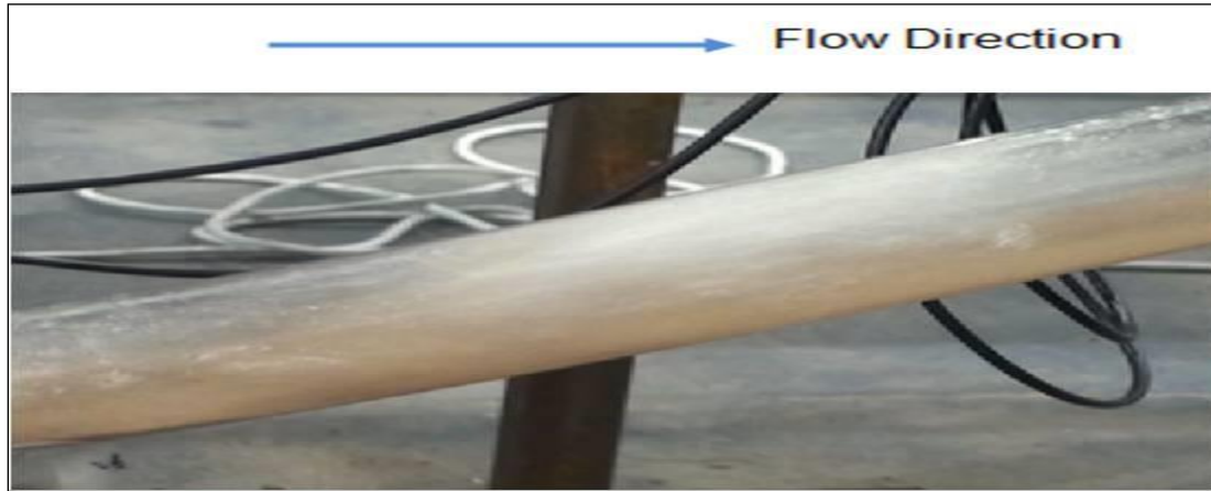
Figure 6-9: Sand transport behaviour before MTC (500lb/1000bbl, V_{sl} =0.08 m/s, V_{sg} = 6.0 m/s)
