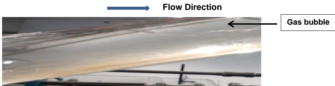
Figure 6-2: sand transport characteristics in plug flow ( V_{sl}=0.55 m/s, V_{sg}=0.2 for 500lb/1000bbl)
