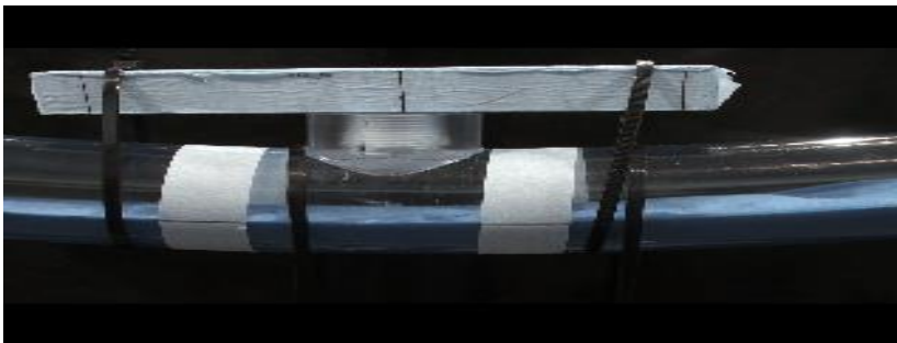
Figure 5-23: Sand bed forming Ripple at water velocity =0.18m/s
