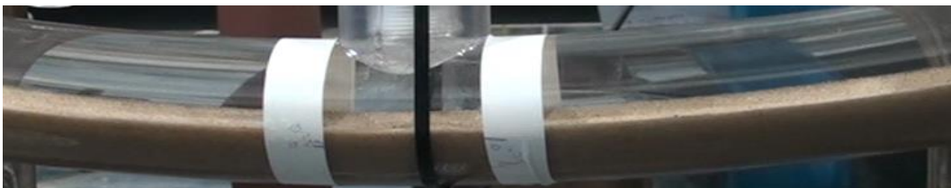
Figure 5-27: 0.44D sand bed layer ( V_L = 0 to 0.20m/s)
