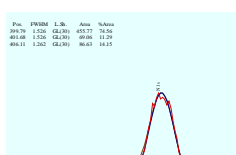
Figure A-5 Carboxylic Dynabeads® Nitrogen subpeaks - N1s (replicate 1).
