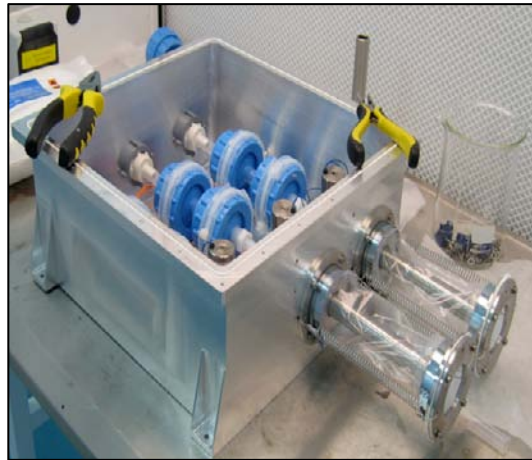
Figure 6-3 UCZ after being assembled inside a cleanroom and before being sealed with a top Tyvek and polypropylene sheet.
