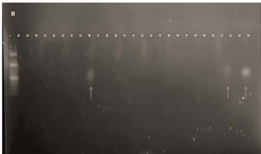
Figure 6-20 Agarose gel with DHMR treated aptamers and SELEX library; i) estradiol aptamer (samples 28 to 30 were at 0.05 \mu\text{M} ; samples 31 to 33 were at 1 \mu\text{M} ; and samples 34 to 36 were at 10 \mu\text{M} ), ii) ibuprofen aptamer (samples 37 to 39 were at 0.05 \mu\text{M} ; samples 40 to 42 were at 1 \mu\text{M} ; and samples 43 to 45 were at 10 \mu\text{M} ), iii) SELEX library (samples 46 to 48 were at 0.05 \mu\text{M} ; samples 49 to 51 were at 1 \mu\text{M} ; and samples 52 to 54 were at 10 \mu\text{M} ), the three buffers were tested at each concentration of each aptamer and library.
