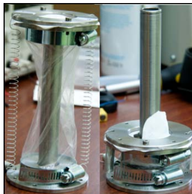
Figure 6-6 Re-designed biobarrier prototype breached by burn wire
