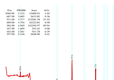
Figure A-1 XPS spectra of 5 \beta -cholanic acid immobilised via cadaverine on carboxylic Dynabeads® surface (replicate 1).
