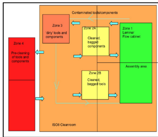
Figure 6-8 Cleanroom organisation diagram of working areas and their degree of cleanliness, from red (less clean) to green (cleaner).
