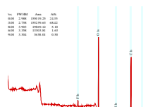
Figure A-15 XPS spectra of carboxylic Dynabeads® immobilised with lysine (replicate 1).
