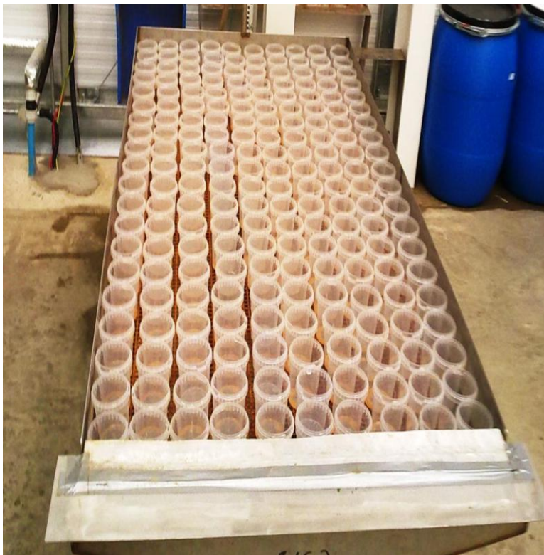
Figure A.1 The erosion rig with 200 plastic cups to calibrate rainfall intensity
