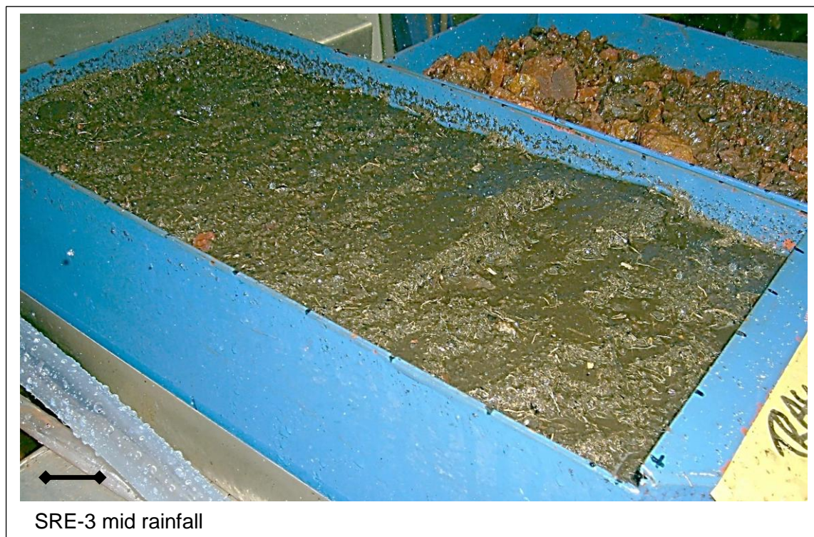
Figure 4.8. SRE saturated after approximately 20mins of rainfall (Scale 1 cm = 3 cm)
