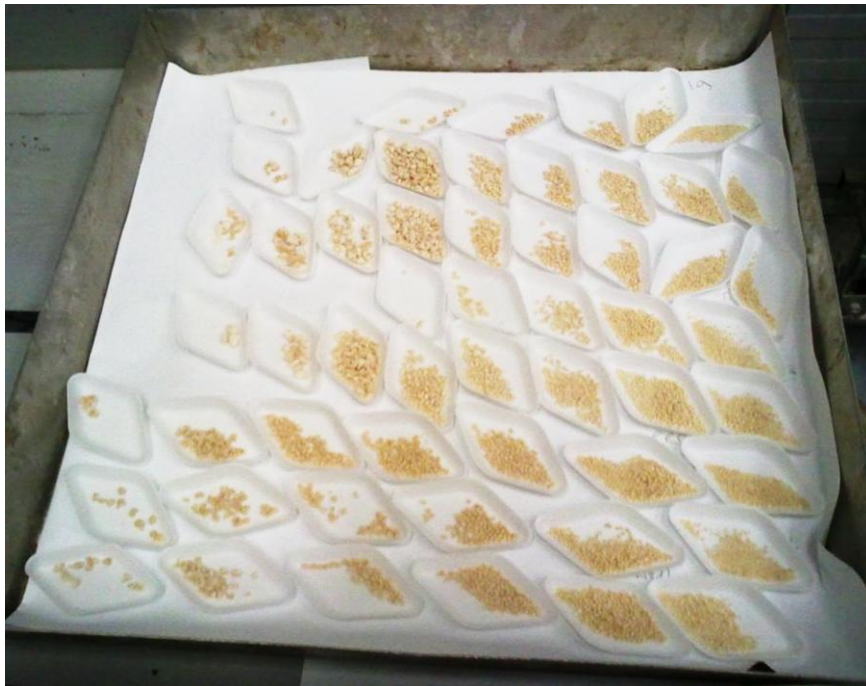
Figure A.3 Different sized flour casts of simulated rainfall made during the rainfall calibration process
