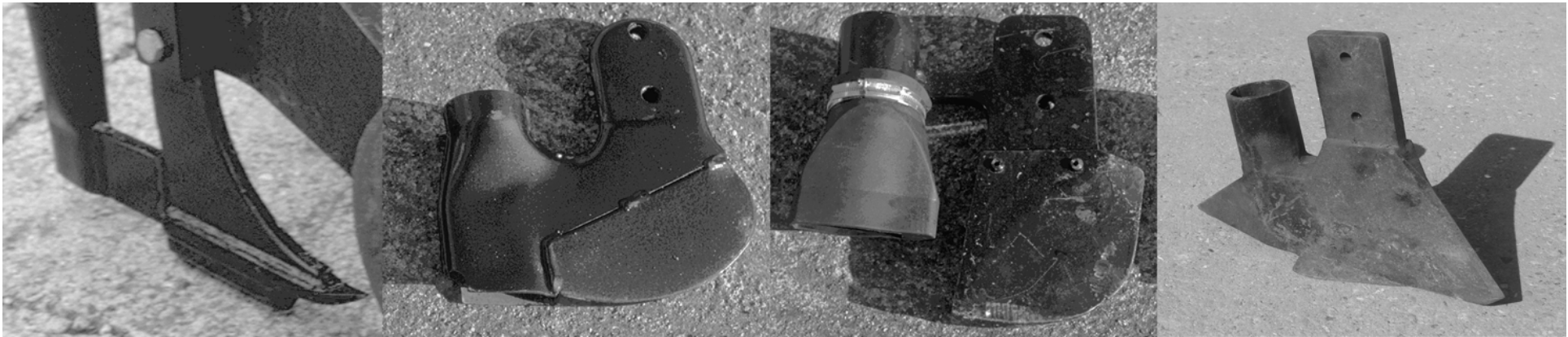
Fig. 7. Commercial injector tines: (a) slipperfoot (C1); (b) shallow I (C2); (c) shallow II (C3); and (d) winged foot (C4)
