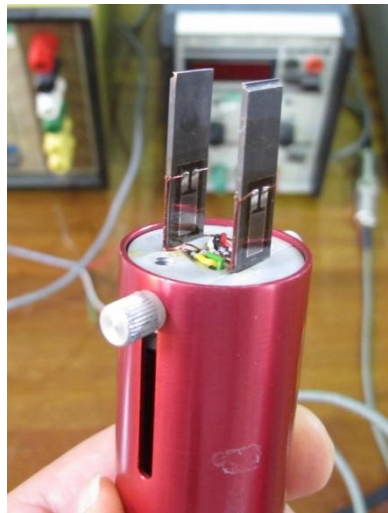
Figure F-1 A customised clip gauge
