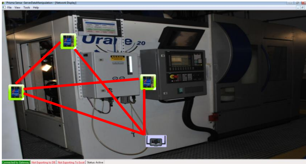
Figure 43: Connection between wireless sensor nodes and gateway. The lines indicate Zigbee connection
