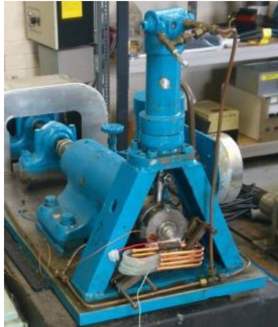
Figure 66: Thermoelectric device and heat sink attached to the casing of the bearings
