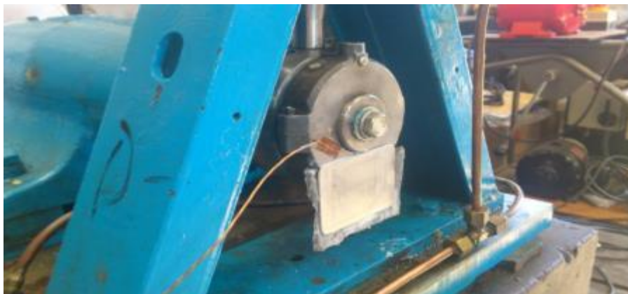
Figure 64: Plate attached to the non-mobile part of the bearing casing
