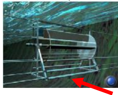
Figure 8: Cross flow turbine by Atlantisstrom [18]
