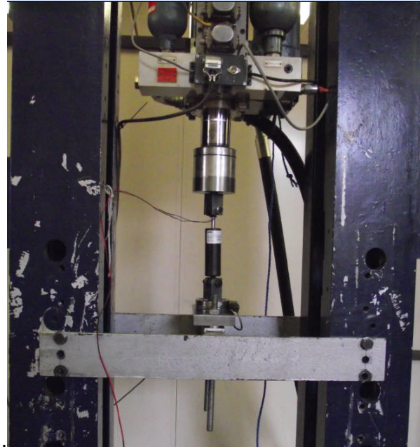
Fig 4.4 Snapshot of MR damper RD8040-1(LORD Corporation) mounted on damper test rig (7 kN/150mmstroke).
