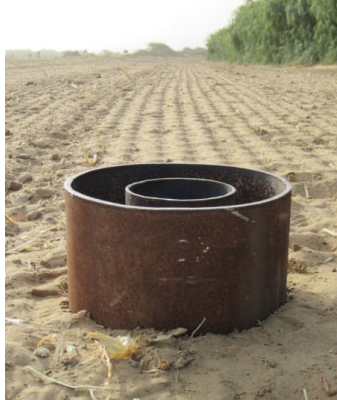
Picture 3.3 Double-ring infiltrometer installed in the farm
