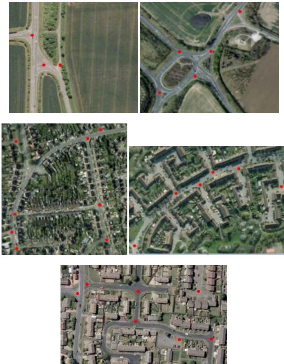
Figure 8-6 road intersection detection results
