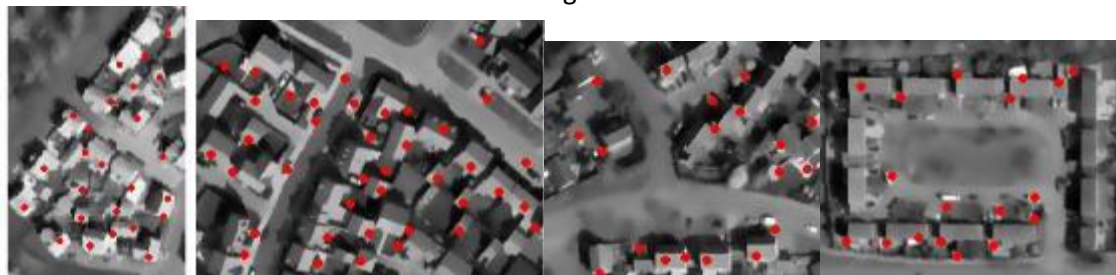
Figure 4-9 Building Detection Results using Harris Corners
