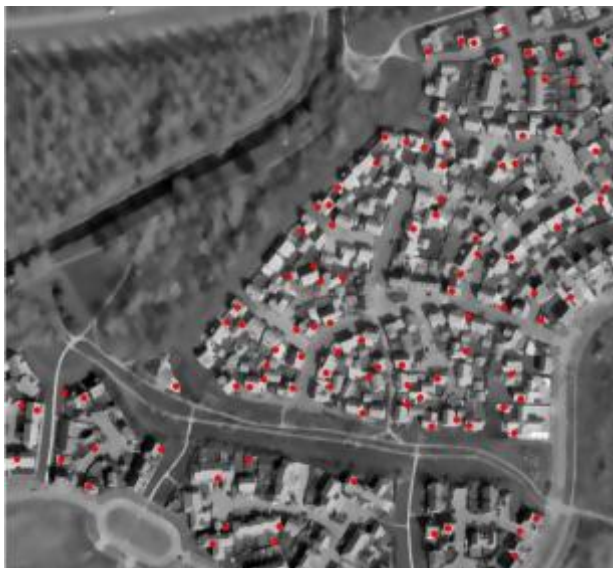
Figure 4-11 Building Detection results using FAST corners
