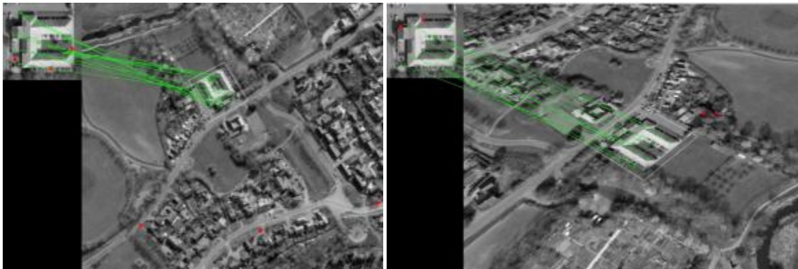
Figure 3-17 SURF rotation and perspective tests show matching can occur at different perspective and rotations
