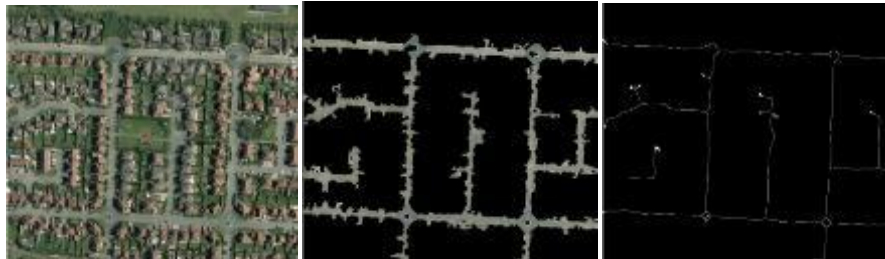
Figure 5-9 Road detection results, original image (right), road regions (centre), road centerlines (left)
