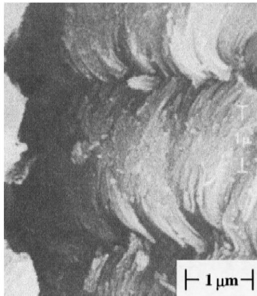
Figure 4.8: SEM of the structure of zirconia columns taken in cross section in the plane perpendicular to the axis of rotation [21]
