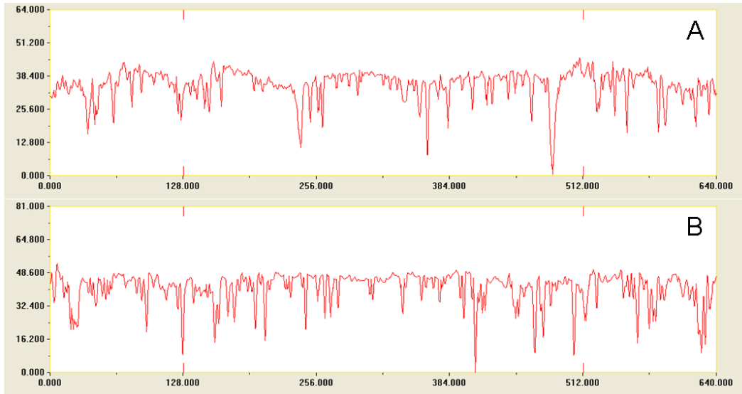
Figure 15.7: Profiles of a 0.05MPa surface (A) and of a 0.4MPa surface (B). The measures are in microns
