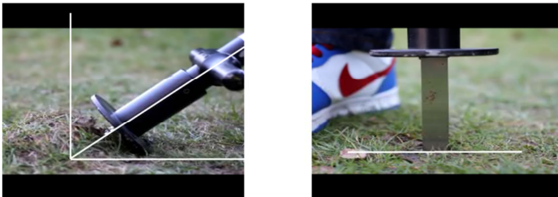
Figure 11-12 Screenshots of videos of the Goingstick shear (left) and penetration (right) movements being analysed.
