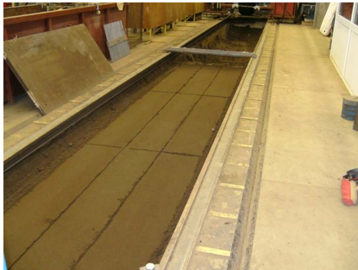
Figure 3-4 Outline of the experimental plot design used in the soil bin. Note that the nearside three plots were not used in the experiment as a result of inconsistent soil conditions produced by a fault with the soil preparation equipment.
