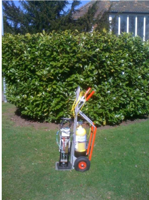
Figure 11-5 The DST device and compressed air cylinder being transported on a sack barrow for use on in-situ surfaces.
