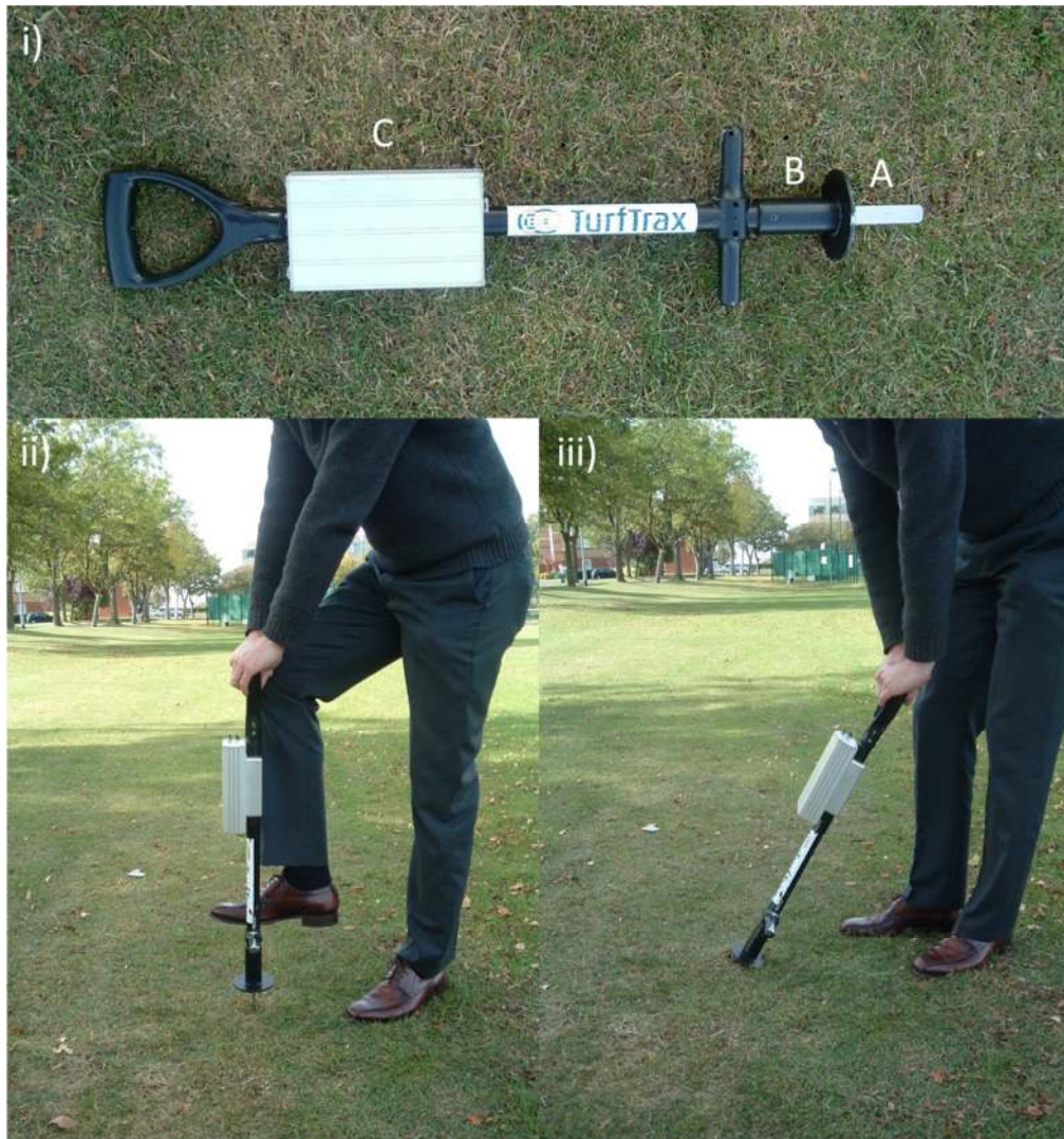
Figure 4-1 i) main components of the GoingStick: tine tip and abutment plate (A), the sensor unit (B), and the signal processor (C); ii) measuring penetration resistance of the surface; iii) measuring shear resistance of the surface.
