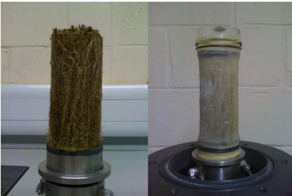
Figure 11-23 Left: a rooted sand soil sample with grass leaves removed; right: a rooted sand soil sample within the rubber membrane prior to testing.
