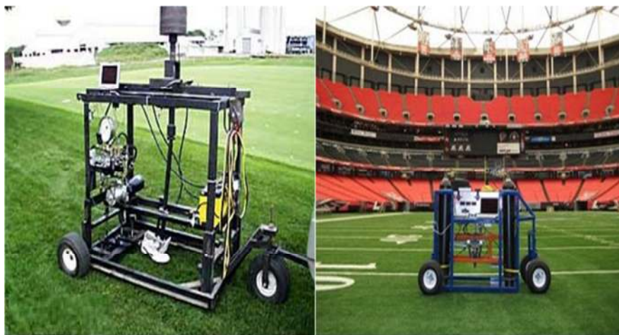
Figure 2-10. Example ‘Category 2’ testing devices measuring traction properties of in-situ surfaces: PennFOOT (left) and the TurfBuster (right).
