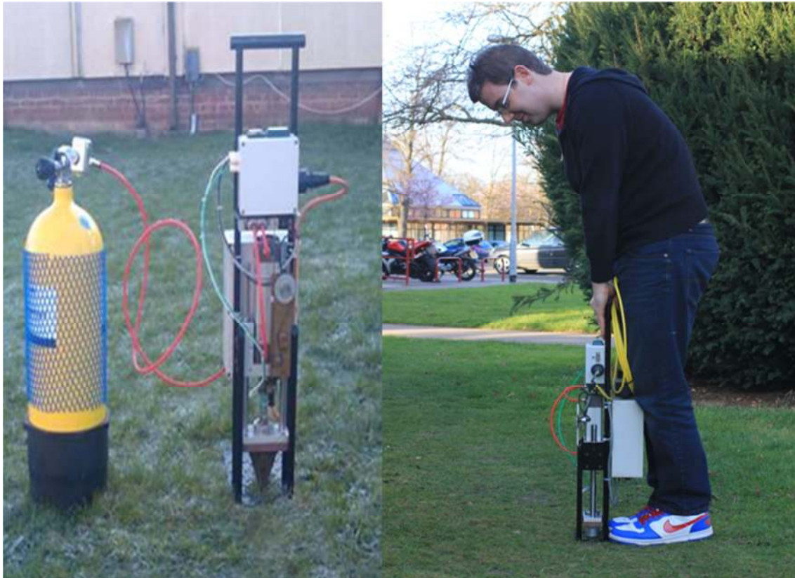
Figure 3-1 Left: The original DST device (with spike test foot), prior to developments made for it to be used on natural turf sports pitches; right: An example of the DST device being used, showing that the operator provides the reaction mass.
