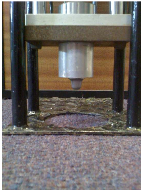
Figure 11-4 Close-up of the studded test foot of the DST device, dimensions 41 mm diameter, 38 mm height, 1320 mm 2 surface area.
