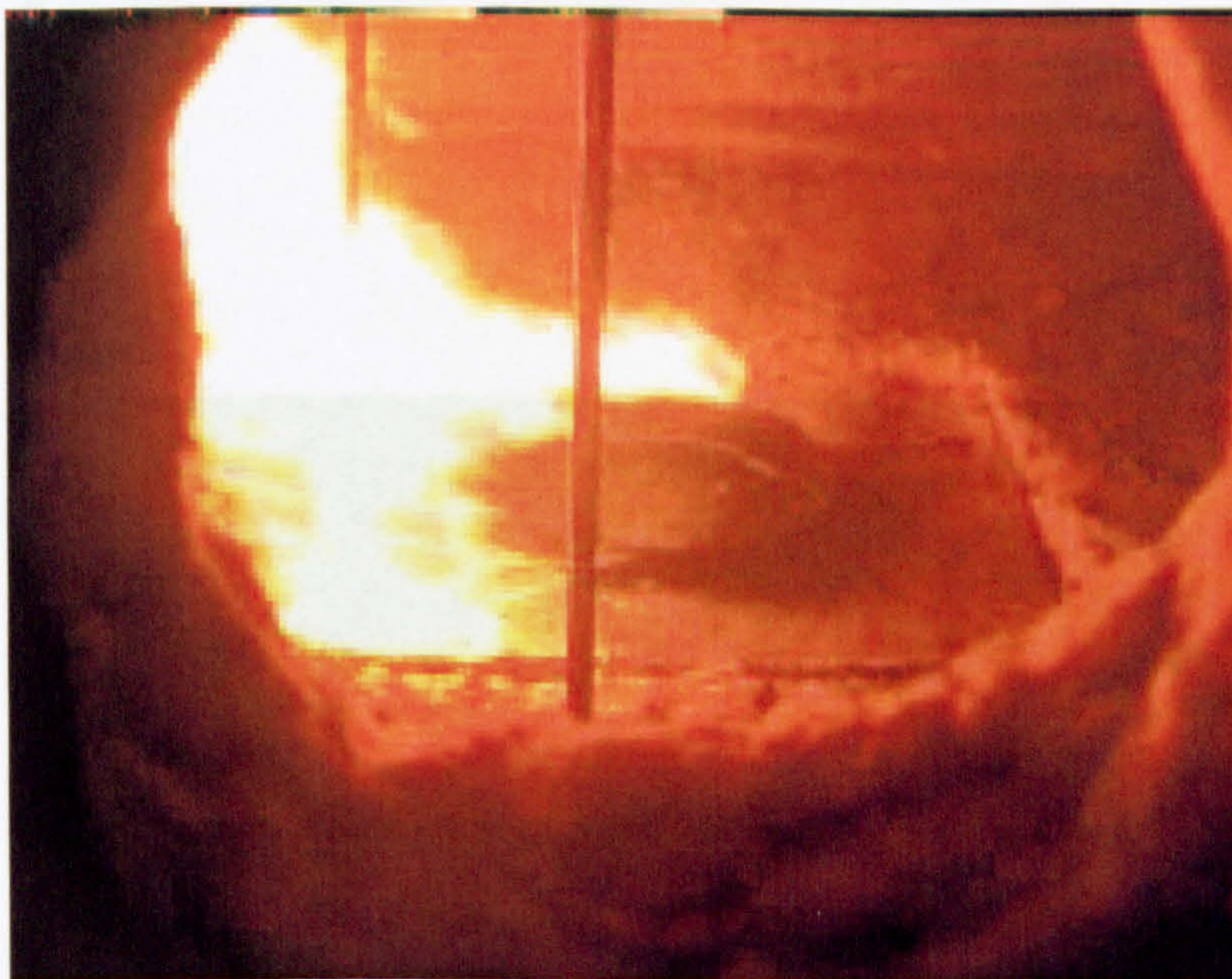
Figure 3.23: Side-view of burner in 0.15m doorwidth configuration showing flame detachment
