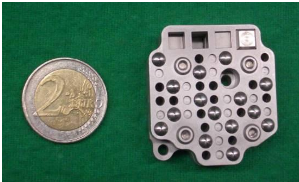
Figure 3-4: A. Design and B. Development Model of the sample holder unit for the LMC on BIOPAN-6 experiment (latter prior to Alodine treatment) (image credits: DLR Germany)
