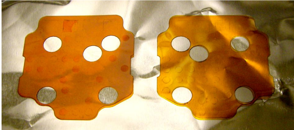
Figure 3-12: Comparison of Kapton foil used in the FM (left) and SC (right) unit. The FM component appeared darker than the SC one in areas unprotected by the metal cover (round spots)
