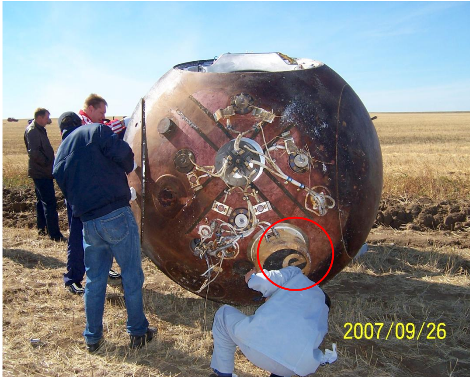
Figure 3-10: FOTON re-entry capsule at the landing site (BIOPAN-6 can be seen in the red circle, bottom centre)
