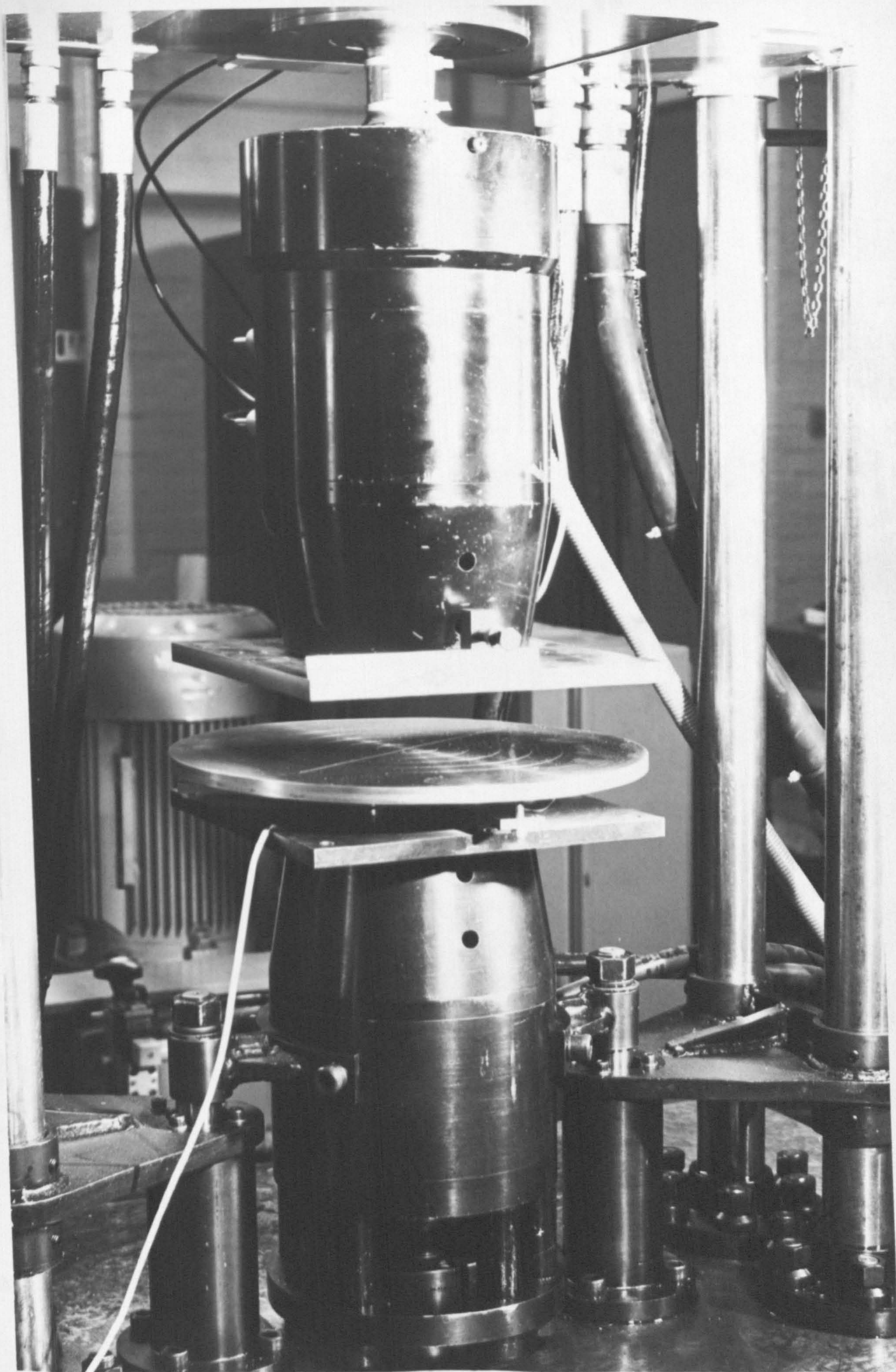
FIG. 4.28 LOAD CELL MOUNTED ON TESTING MACHINE
